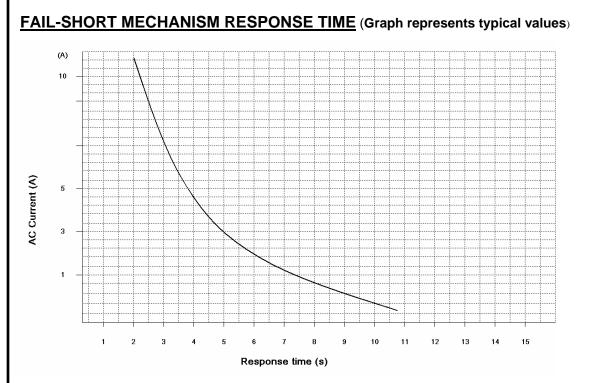
Note: Both electrodes simultaneously powered, each with the AC current value in the graph
